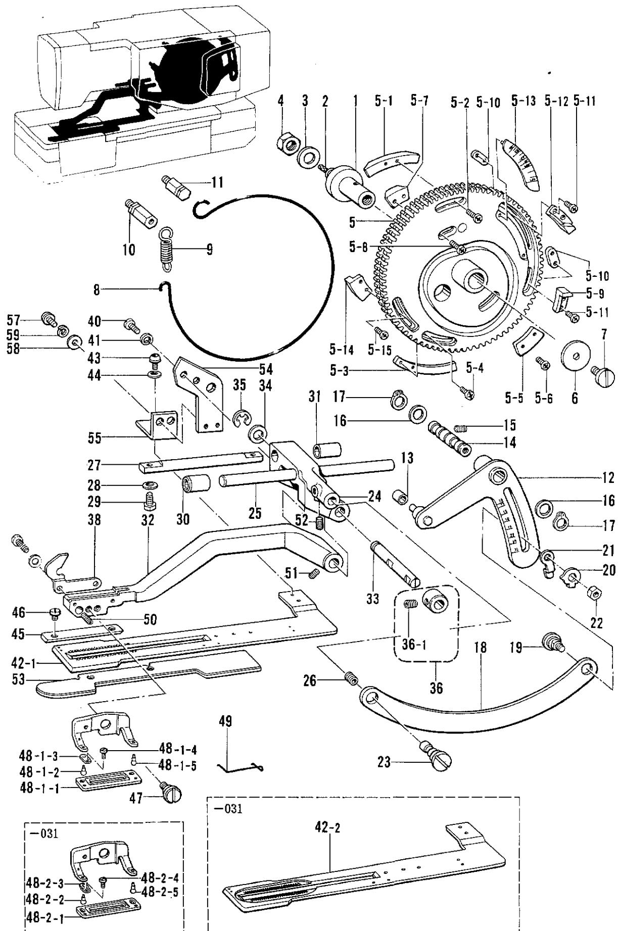
**M. 送り関係/Feed mechanism/Transportvorrichtung/
