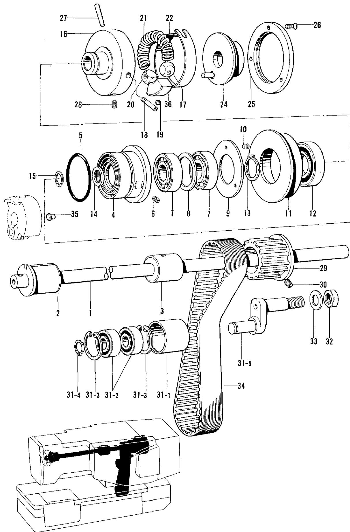
B. 上軸関係/Upper shaft mechanism/Obere Welle/
