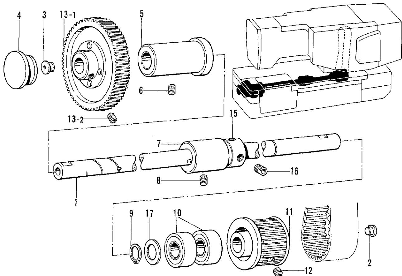
P. 糸切れ感知関係 / Thread breakage detector mechanism / Fadenbruchfühler /
