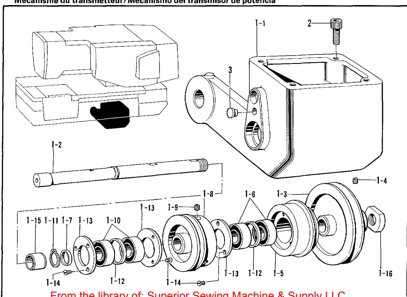
D. 針棒関係/Needle bar mechanism/Nadelstangenvorrichtung/
